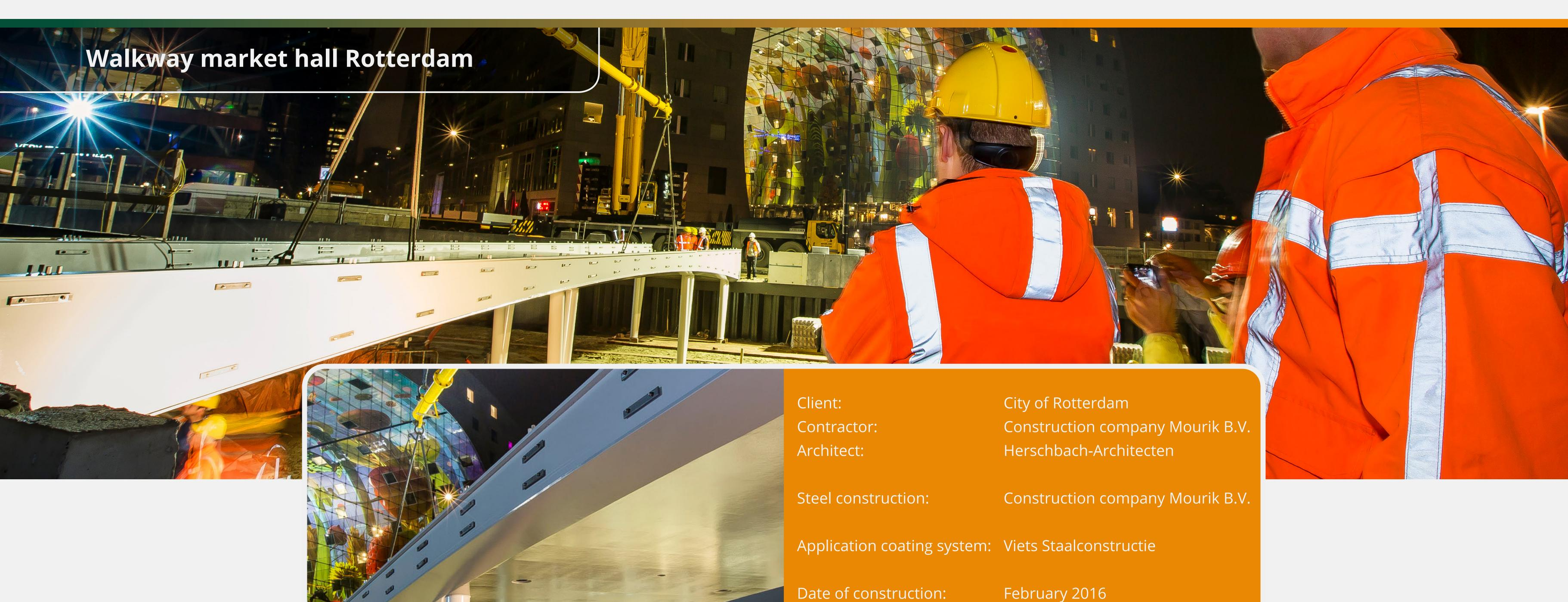
The square in front of the Rotterdam Market Hall has been transformed in 2015, commissioned by the City of Rotterdam. A walkway has been constructed to cross over the deepened bicycle shed, which connects the Blaak with the market. A telescopic crane with a lifting capacity of 400 tons was needed to get the 30-tonne bridge in place. The bridge was finished with natural stone pavement afterwards.
